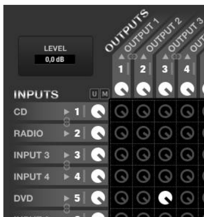
MUTE OFF for input 5 – output 3 (send enabled)
