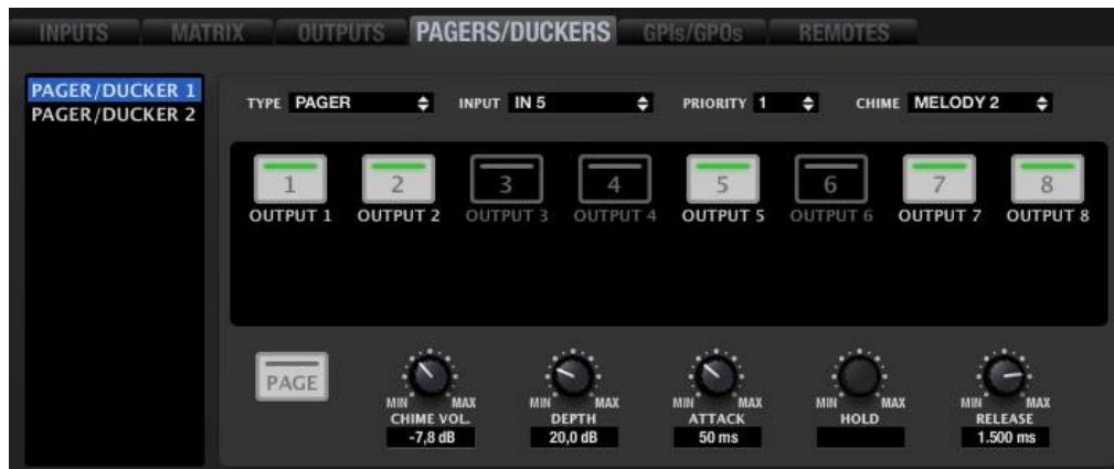
Details of the PAGERS/DUCKERS section from which you configure the operation of an MPAGE16 / eMPAGE unit connected to the system
