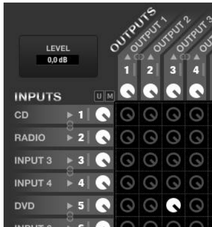
MUTE OFF for input 5 – output 3 (send enabled) MUTE ON for input 5 –output 3 (send disabled)
