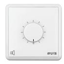
The Aart E-VOL60 is a 100 volt volume control. It can handle up to 60 watts of power. It is very versatile thanks to the step-by-step attenuation in 11 steps + zero position. The E-VOL60 is designed to handle 24V priority signals. This means that you can always get an announcement out, even to zones where the local volume control is in the 'OFF' position!
